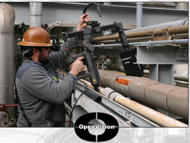
OpenVision<sup>TM</sup> live video x-ray system enables real time, qualitative screening for corrosion under insulation (CUI). CUI causes unscheduled downtime if not identified and corrected, posing major cost and safety issues. Identify problem areas quickly, saving valuable time and resources. Scan miles with OpenVision<sup>TM</sup> versus mere feet accomplished by other NDT methods.
